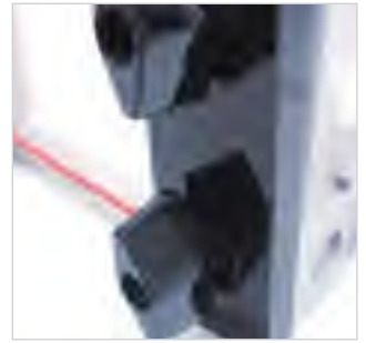
03. Robust side clamps hold the gel in place
